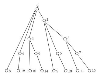
Figure 2: Broadcasting tree of machine 0 with 4 rounds starting at round 0.
