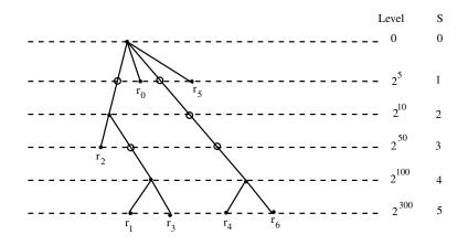
Figure 1: Real numbers are inserted according to Algorithm Insert. Circled position has no number inserted. Dotted position has integer and/or real number inserted. Real numbers are inserted at leaves.
